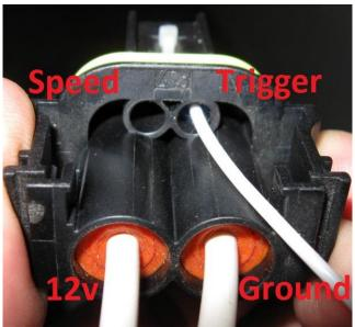
Figure 7 - Fan plug wiring
