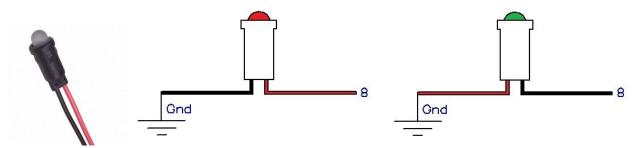
Figure 3 - Installing the Remote Status LED to operate either Red or Green
