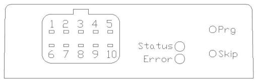
During programming, the fan will turn off to allow the engine to warm up faster. Press and hold **Prg** until the Status LED lights with the color of the sub-menu you wish to enter, then release **Prg**. Holding **Skip** for 4 seconds will exit any programming menu and return the controller to normal operation. Details about each programming sub-menu can be found on the next page. The Status and Error LEDs will change colors to indicate the current location in the programming flowchart.
