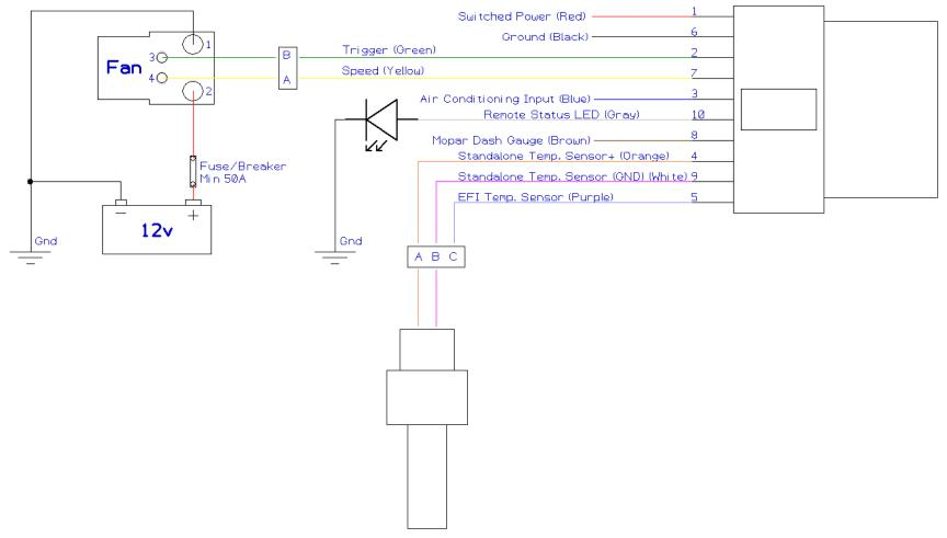
Figure 5 - Wiring with a two terminal temperature sensor installed
