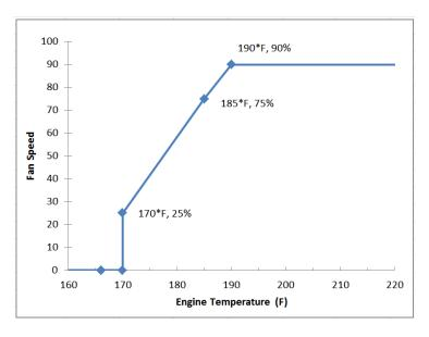
Figure 1 - Fan speed vs. Engine Temperature
