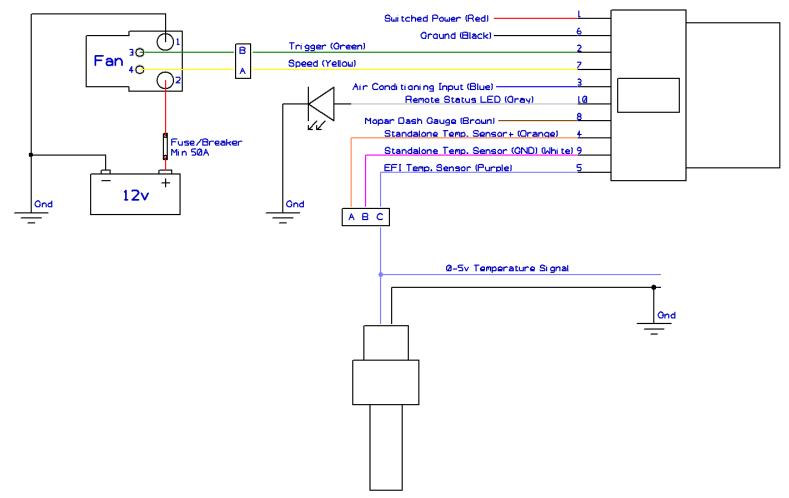
Figure 6 - Wiring using a 0-5v EFI temperature sensor
