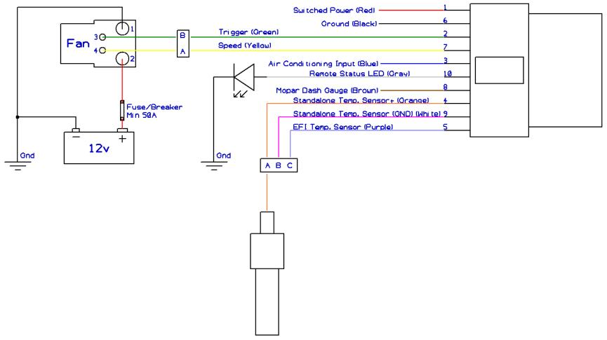
Figure 4 - Wiring with a one terminal temperature sensor installed
